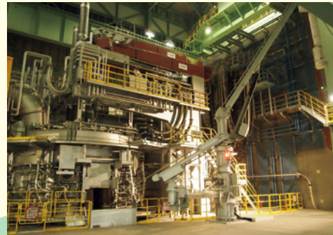
Electric arc furnaces with rotating drives "STARQ®"
