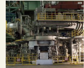
The 150t furnace (STARQ ® ) introduced at the Chita Plant
