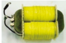
3 kW class reactor
