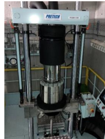
High-pressure hydrogen gas atmosphere furnace materials testing machine (Outside pressure type)
