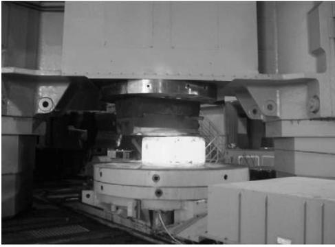
Fig.13. SUS304N2 disk under forging.
