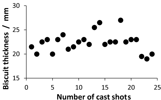
Fig. 9. Fluctuation of biscuit thickness during production. The sprue core is made of steel B.
