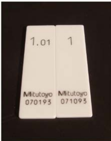
Fig. 4. Standard gauge. (thickness 1.01 mm and 1.00 mm)
