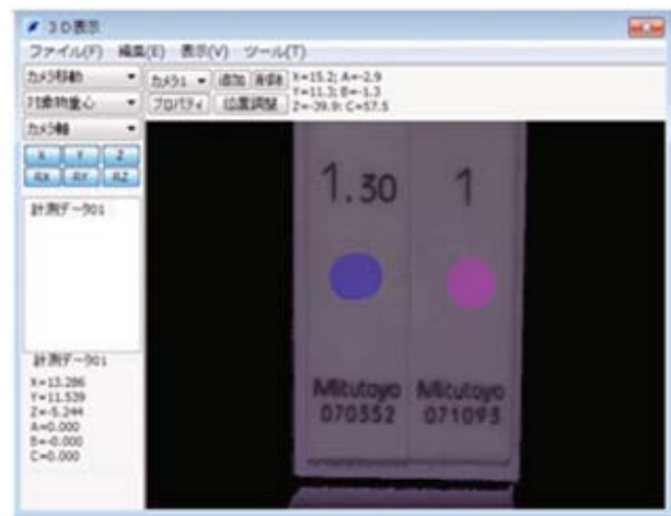
Fig. 19. Vertical distance measurement using plane fitting.
